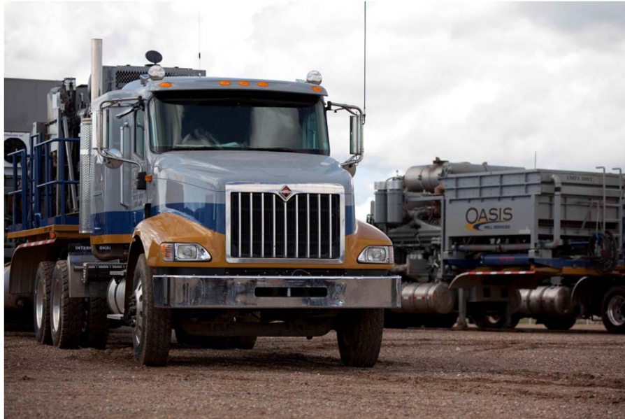
OWS Hydraulic Pumping Unit
